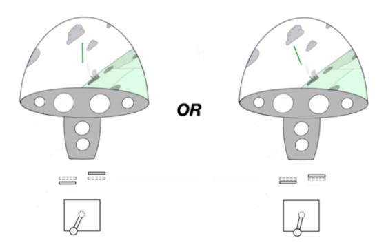
The first drawing shows the string in the middle and the positions of stick and rudder required to achieve this: a considerable amount of right rudder with a lot of back stick and out-of-turn aileron. The controls are crossed, but this is safe and normal in a glider as long as the yaw string isn't pointing into the turn.
